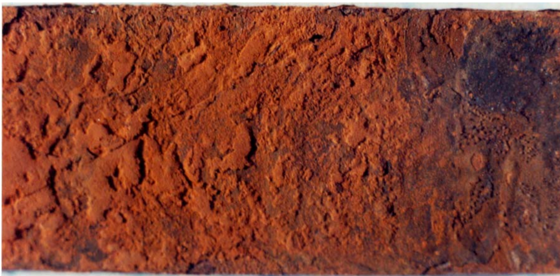
CLOSE UP PHOTO OF CORROSION COUPON, OZONE/SOFT WATER
