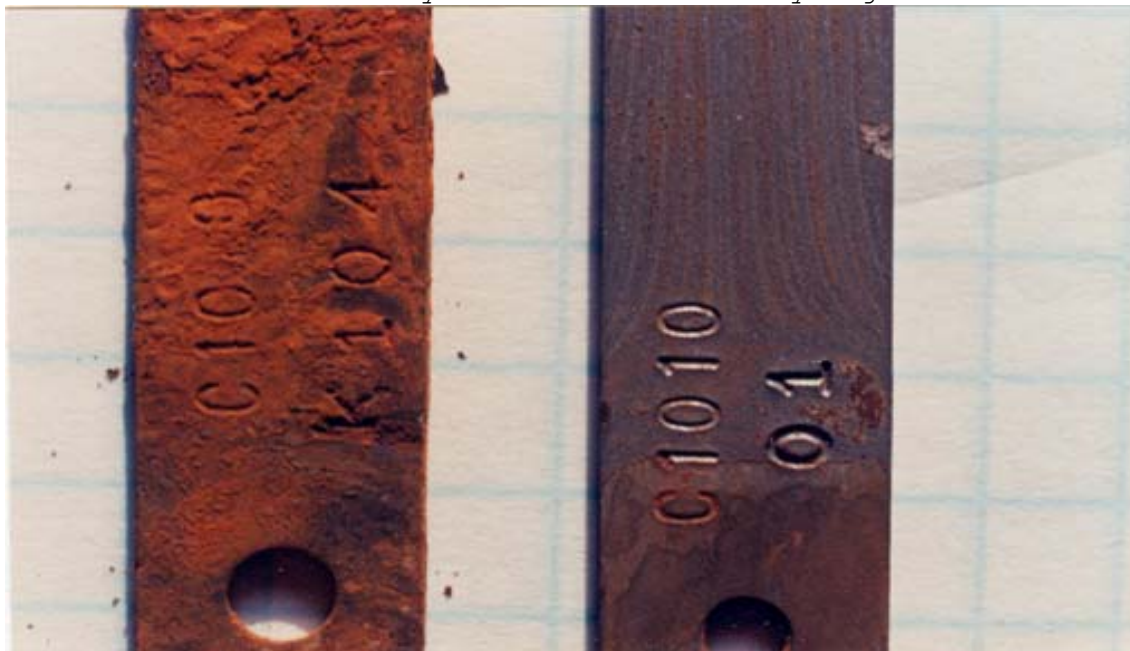
COUPONS FROM OZONE AND CHEMICALLY TREATED SYSTEMS
