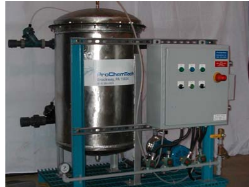
Skidded automatic sand filter
